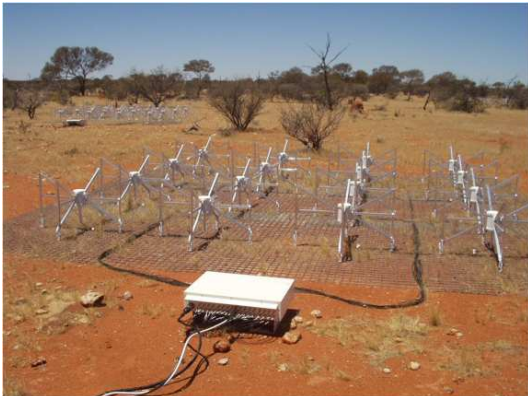
FIG. 5: MWA antenna tile ( 5\text{m} \times 5\text{m} ), consisting of 16 broadband, crossed dipoles with low-noise amplifiers in central hub. Signals are routed to the adjacent analog beamformer; power and coaxial cables to the digital receiver exit at the bottom [13].
