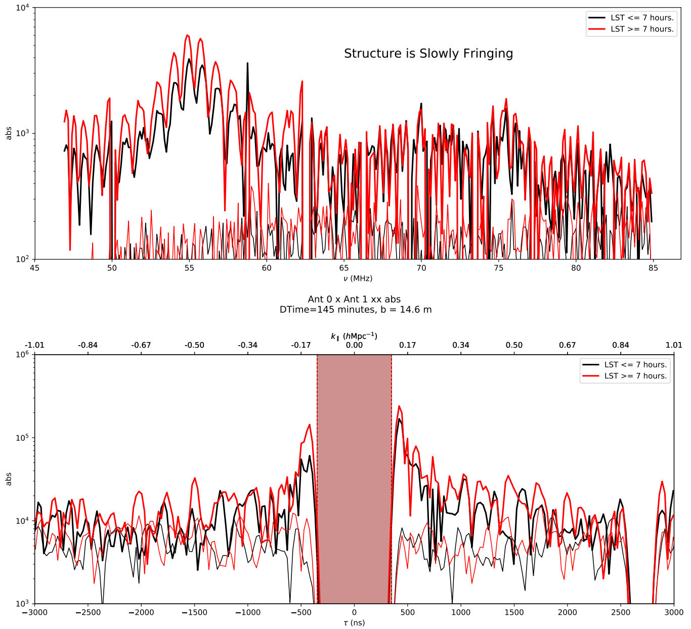
Figure 14. Top: A comparison of residuals from two coherent integrations, each over \sim 2 non-overlapping hours of LST. The high-delay residuals agree very well, suggesting further that they arise primarily from low delay-rate sources (instrumental or otherwise).
