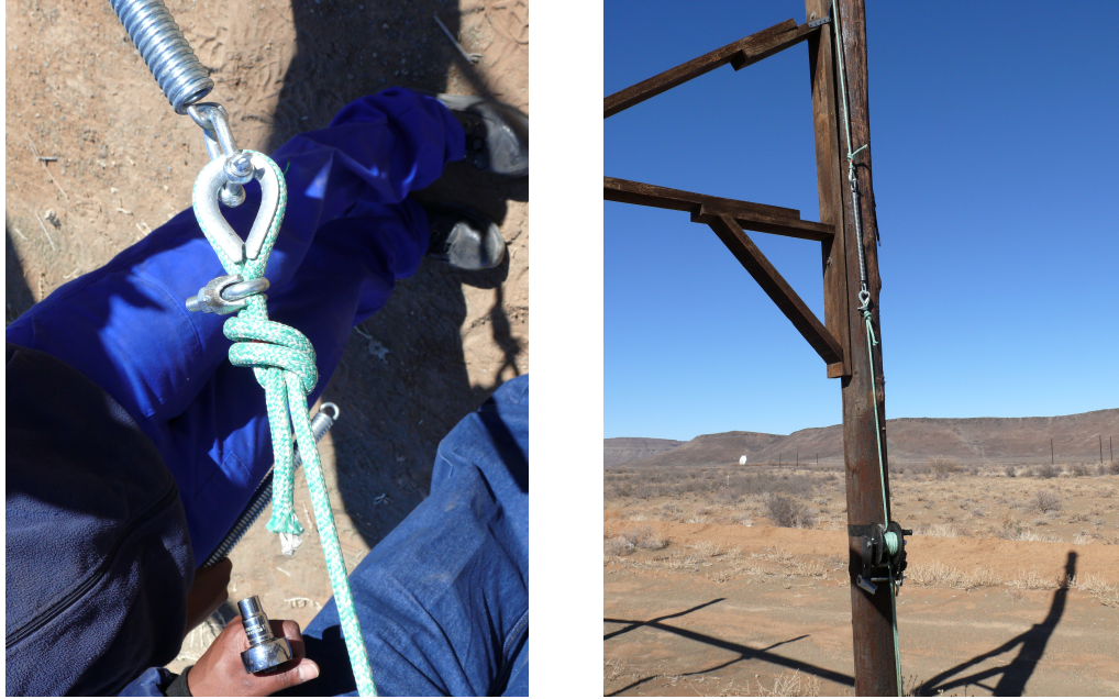
Figure 16. Left panel: A picture of the lifting line - spring attachment for the ‘springs in series’ approach. A double overhand knot with a good-sized tail is tied; the thimble is inserted, and the saddle clamp is used to hold the rope together so the thimble does not fall out. Right panel: A picture of the lifting line with a spring attached in series. This was taken during the July-Aug 2019 site visit.
