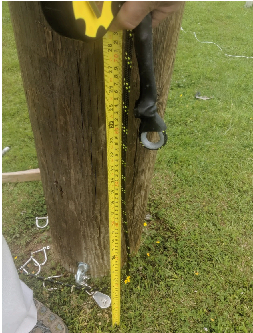
Figure 15. Positioning the feed end and winch end of the lifting line to determine where to cut for spring placement. The line goes from the thimble, through the top pulley, and then drops back to the ground. For the spring in series with the line: If the thimble is positioned 72 cm above the ground, the location to cut is also 72 cm above the ground. Note that the image shows 60 cm; this was for the saddle clamp approach that is not being pursued. The line should be pulled tight when measuring. Attaching a light line to the thimble prior to taking the thimble out of the dish makes it much easier to reattach the thimble to the feed.
