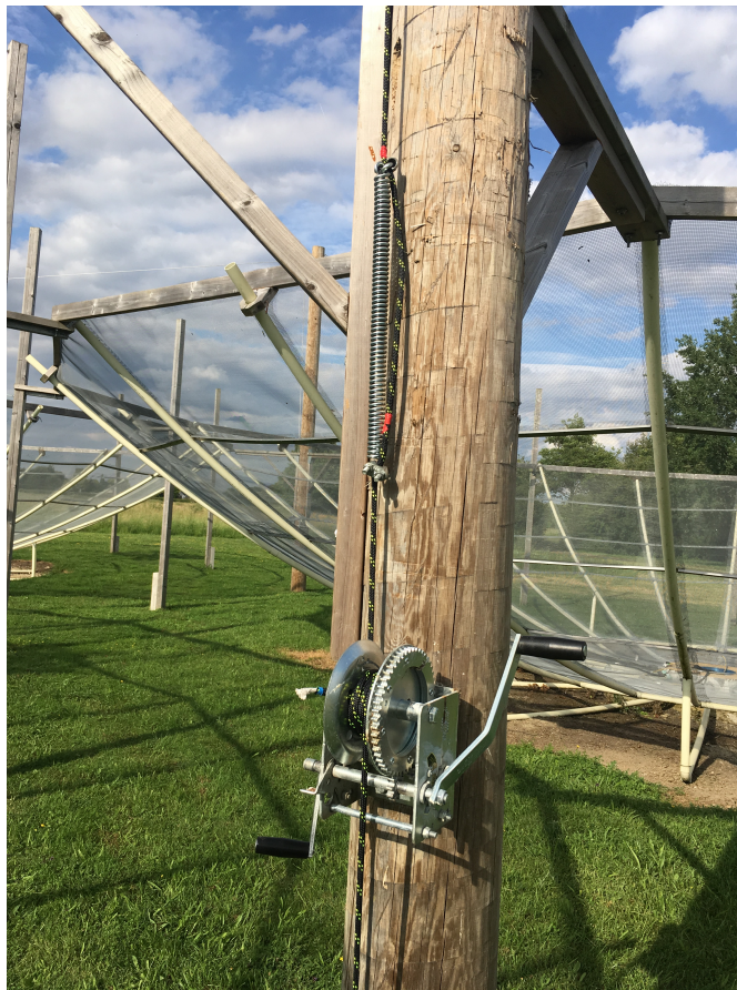
Figure 10. A picture showing the approach of the spring in parallel with the line. Here the length of line between the top and bottom saddle clamps is 48 cm; the photo shows that there is still a little slack in the line when the feed is in position.
