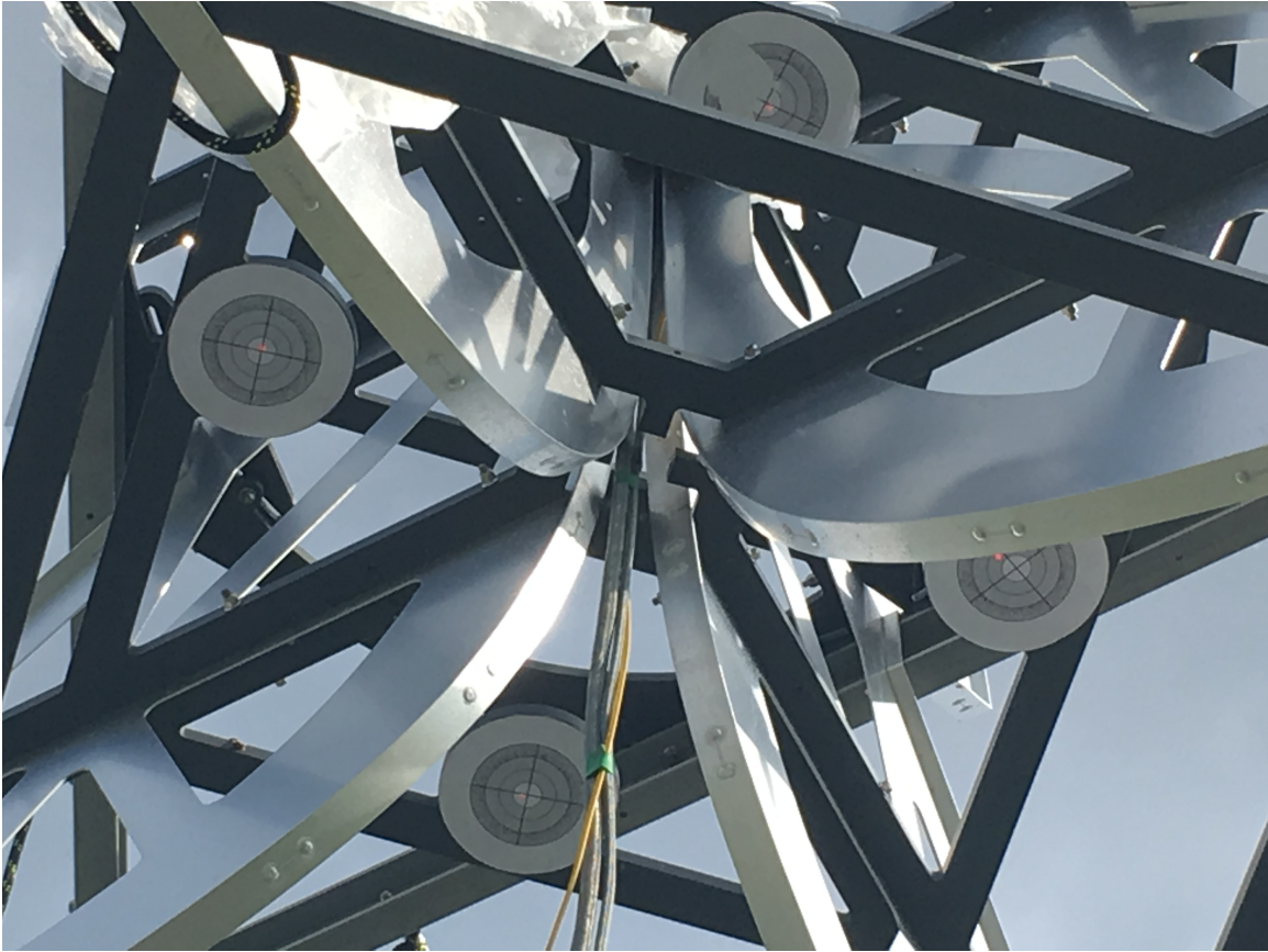
Figure 9. A picture showing the upward laser beams from the plumb-bobs and the distance measure shown in the first picture. The right-most circle shows the laser measure beam, which is used only for the z measure. The other circles show the (fainter) beams of the plumb-bobs, all very near the centers of the concentric circles. The diameters of the innermost circles differ by 2cm, so the distance between each line radially is 1 cm. Note that the beams indicate that a better match to the centers would be had by rotating the plywood clockwise about the z axis. For this positioning the x-y positions are all well within a cm of their desired location, and the z measure is exact to the precision of the laser measure: 4.427 meters. This measure takes into account the 11mm thickness of the plywood.
