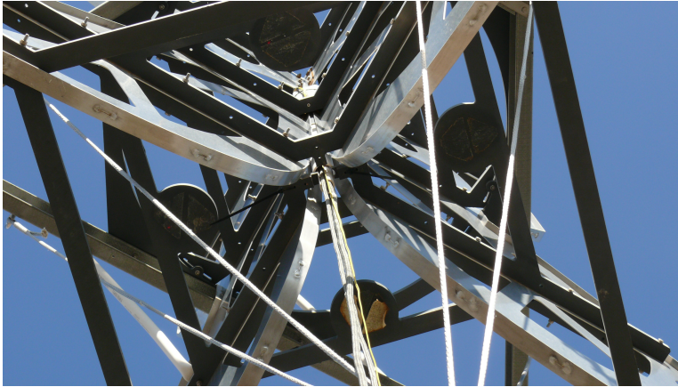
Fig. 1.— A HERA feed viewed from below. The conduit is in the cavity formed by the four feed blades, and three cables can be seen emerging from the bottom of the conduit.
