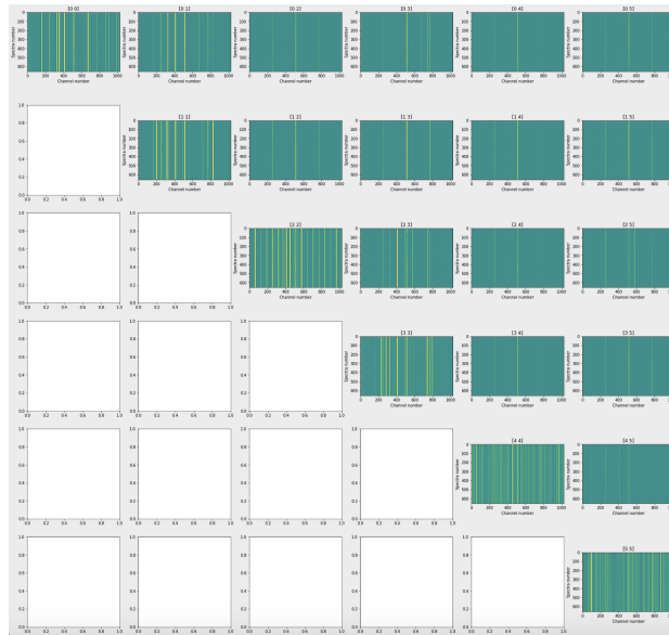
Figure 14: 1 hr integration waterfalls for the 08-2019 Fengine. Off diagonal correlation is clearly seen.
