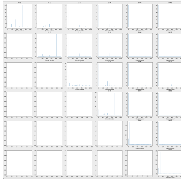
Figure 1: The correlation matrix for the 08-2019 Fengine. The row and column designation determine the input number to the snap (in order of the hera_corr_f correlator numbering), making the diagonal axis the autocorrelations and all other correlations numbered respectively. Off diagonal correlations are expected to be close to -70 dB down if there is not excess correlation.
