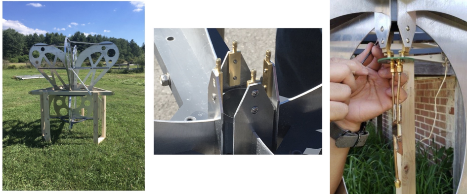
Fig. 1.— Left: A HERA Vivaldi feed, inverted for on-sky testing at Green Bank in July 2018. Center: Detail of the four-pin feed point assembly. Right: The assembly of the feed points, custom adaptor plate, and Macom HH-128 180-degree hybrid as a balun.
