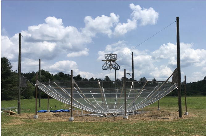
Fig. 2.— The Vivaldi feed on the HERA dish in Galford Meadow.
