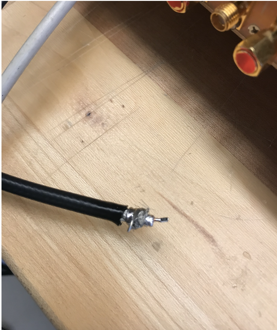
Figure 1: An image of the homemade sniffer probe used to make measurements of the clock line
