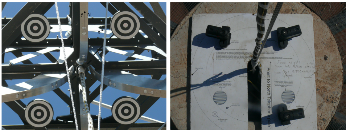
Figure 2: Left: An example of the photos used to determine the x and y feed displacements for a single antenna. Right: The plywood jig centered over the hub of the antenna's dish. The laser points seen on the targets in the left photo are produced by laser plumb-bobs attached to the jig. If the feed is perfectly centered in x and y , the laser points should appear in the centers of the targets. We can identify north (+ y ) by the metal arm which is flanked by two white ropes on either side.
